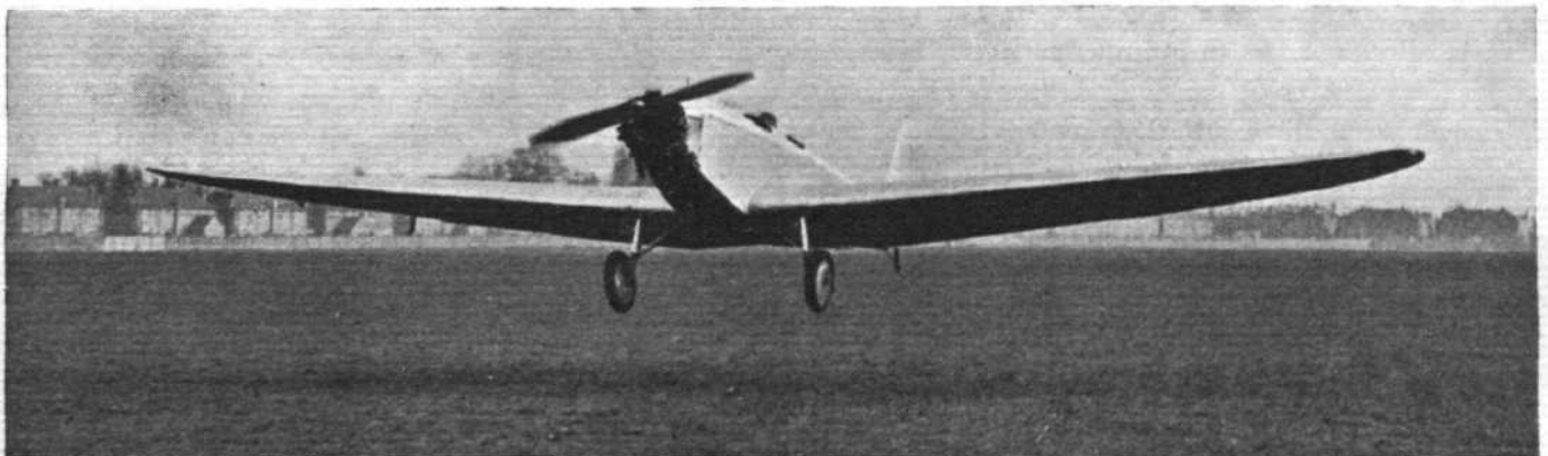
A CLEAN FRONT: Large wing area and low wing loading give this Pobjoy-engined British Klemm "Swallow" a spectacularly low landing speed. (FLIGHT Photo.)
